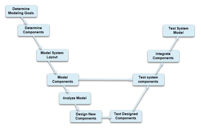
The workflow in this tutorial focuses on fundamental Simulink tasks as they relate to Model-Based Design.
