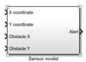
2 Construct the distance measurement subsystem. In the Sensor model block, use Subtract, Math Function with function magnitude^2, Sum, and Sqrt blocks as shown. Note the reordering of the input ports.
