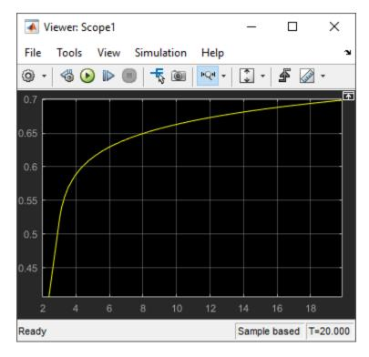
At time 3, the position of the robot is at about 0.55 m. When the simulation ends, the position is less than 0.71 m. It is safe to say that the robot travels less than 0.16 m after the power is cut.
