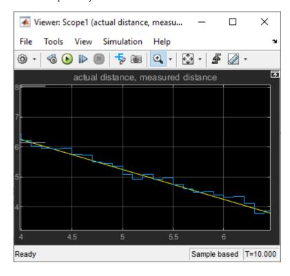
From the plot, note that the measurement can deviate from the actual value by as much as 0.3 m. This information becomes useful when designing a safety feature, for example, a collision warning.
