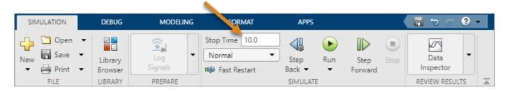
The default stop time of 10.0 is appropriate for this model. This time value has no unit. The time unit in Simulink depends on how the equations are constructed. This example simulates the simplified motion of a car for 10 seconds — other models could have time units in milliseconds or years.
