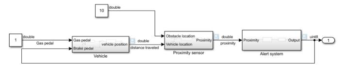
The model displays data types along the signal lines. Most signals are double, except the output of the Alert system. Double-click the subsystem to investigate.
